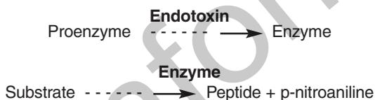
The Endosafe® -PTS cartridge and its interface with the reader have been designed to mimic currently licensed Endpoint Chromogenic and Kinetic Chromogenic Methods by measuring color intensity directly related to the endotoxin concentration in a sample. Each cartridge contains precise amounts of FDA licensed LAL formulations, chromogenic substrate, and Control Standard Endotoxin (CSE).
