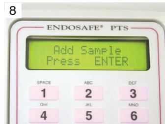
8 Once the reader displays “Add Sample Press ENTER” the assay is ready to be initiated. Press “Enter”. After assay is complete, results appear on screen. Data can be printed or downloaded to computer.
