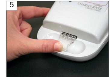
5 Insert cartridge firmly into the slot at the front of the reader with the sample reservoirs facing up.
