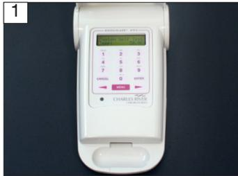
1 Press the MENU key on the PTS<sup>™</sup> to turn the reader on. The reader begins a “System Self Test” and heats to 37°C in approximately 5 minutes.
