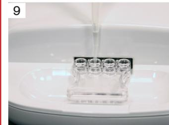
9 Holding the pipette straight up and down at the bottom of the sample well can force some sample into the channel early and disrupt the reagent mixing stations. Avoid any technique which is prone to splash out or bubbles.
