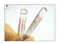
Record results: + if firm gel, - if no firm gel; PPC must gel for test to be valid.
