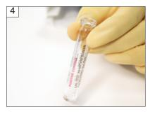
Aseptically add 0.2 mL of sample into red cap PPC assay tube; gently mix.
