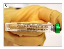
Incubate for times indicated on vial label (+/- 2 minutes); timing is critical.
