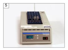
Immediately place reaction tubes in 37°C dry bath or water bath.
