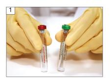
Gently tap the bottom of the LAL and Positive Product Control (PPC) and Single Test Vials (STV) on hard surface.
